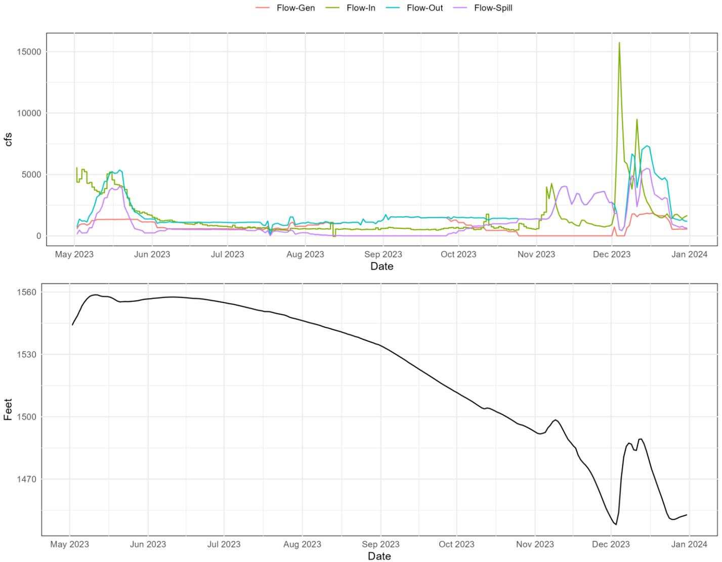
**Figure 14.** Dam operations at Detroit Dam. Top panel presents flow through the powerhouse (Flow-Gen), flow into the reservoir (Flow-In), flow out of the reservoir (Flow-Out), and flow through the spill gates (Flow-Spill). The bottom panel presents the forebay elevation.
