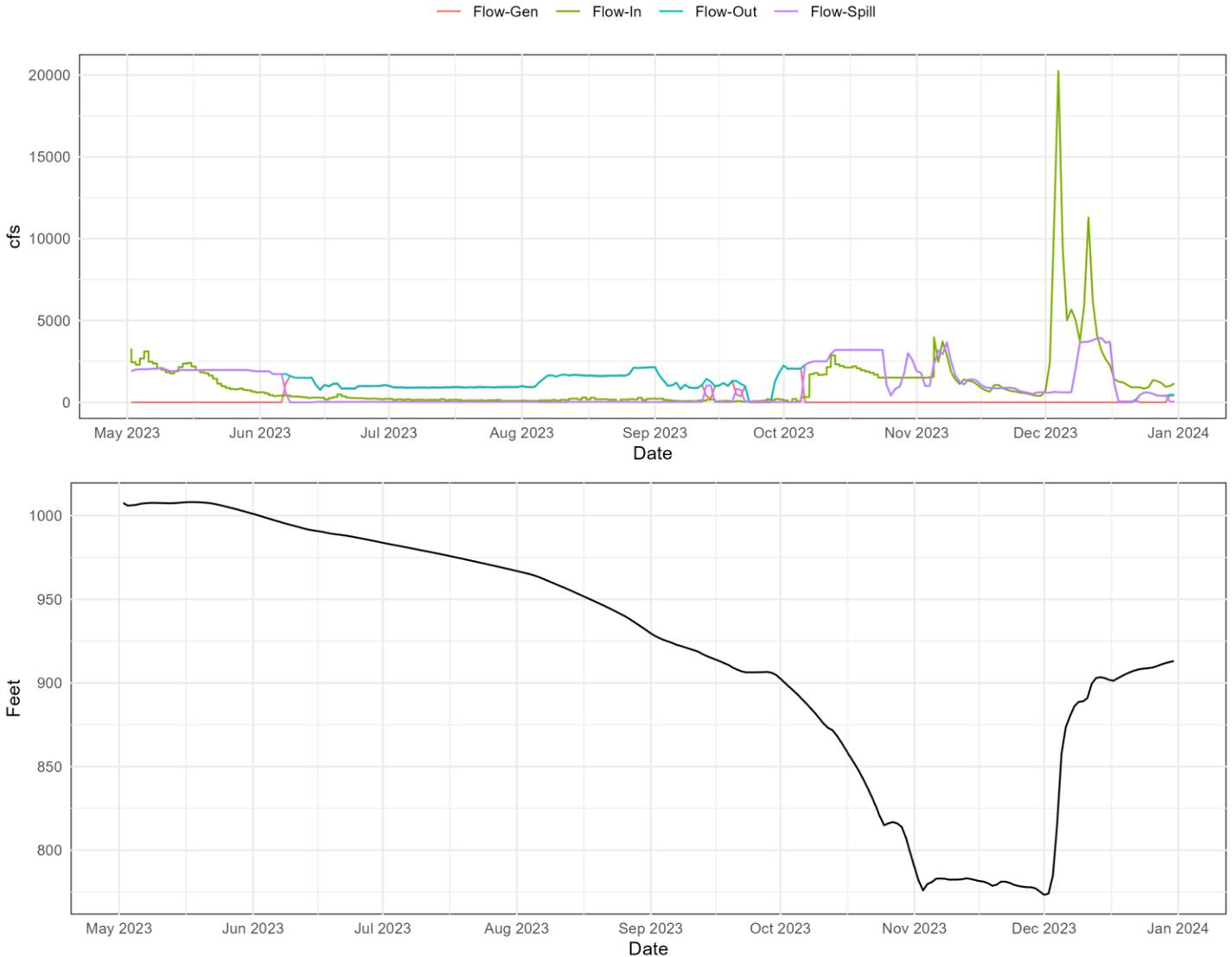
**Figure 12.** Dam operations at Green Peter Dam. Top panel presents flow through the powerhouse (Flow-Gen), flow into the reservoir (Flow-In), flow out of the reservoir (Flow-Out), and flow through the spill gates (Flow-Spill). The bottom panel presents the forebay elevation.
