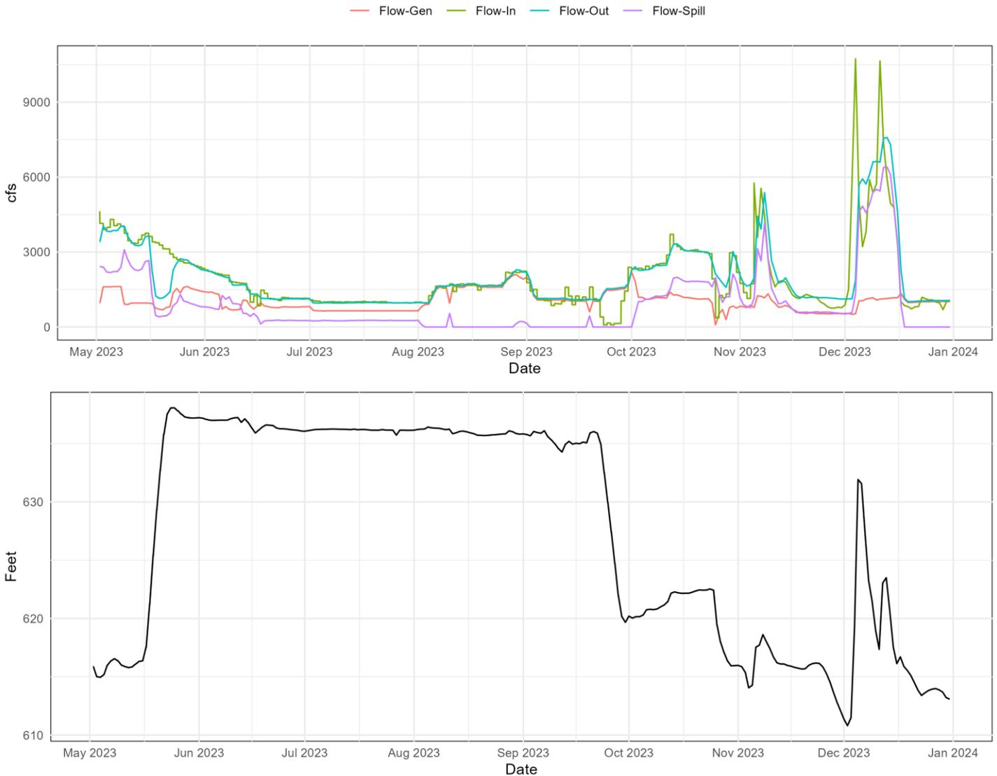
**Figure 13.** Dam operations at Foster Dam. Top panel presents flow through the powerhouse (Flow-Gen), flow into the reservoir (Flow-In), flow out of the reservoir (Flow-Out), and flow through the spill gates (Flow-Spill). The bottom panel presents the forebay elevation.
