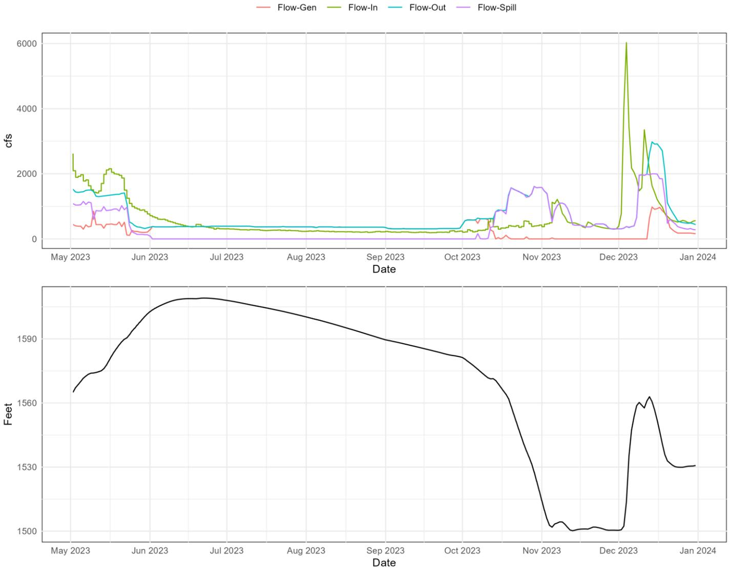
**Figure 8.** Dam operations at Cougar Dam. Top panel presents flow through the powerhouse (Flow-Gen), flow into the reservoir (Flow-In), flow out of the reservoir (Flow-Out), and flow through the regulating outlet (Flow-Spill). The bottom panel presents the forebay elevation.
