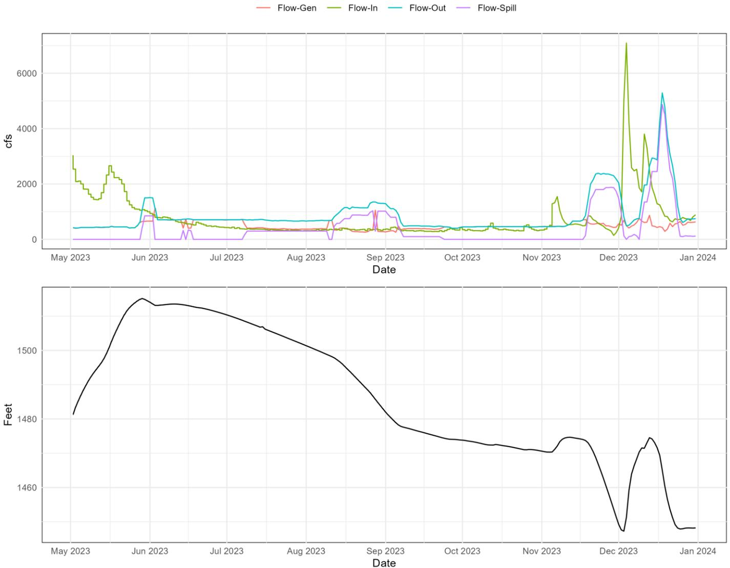
**Figure 9.** Dam operations at Hills Creek Dam. Top panel presents flow through the powerhouse (Flow-Gen), flow into the reservoir (Flow-In), flow out of the reservoir (Flow-Out), and flow through the regulating outlet (Flow-Spill). The bottom panel presents the forebay elevation.
