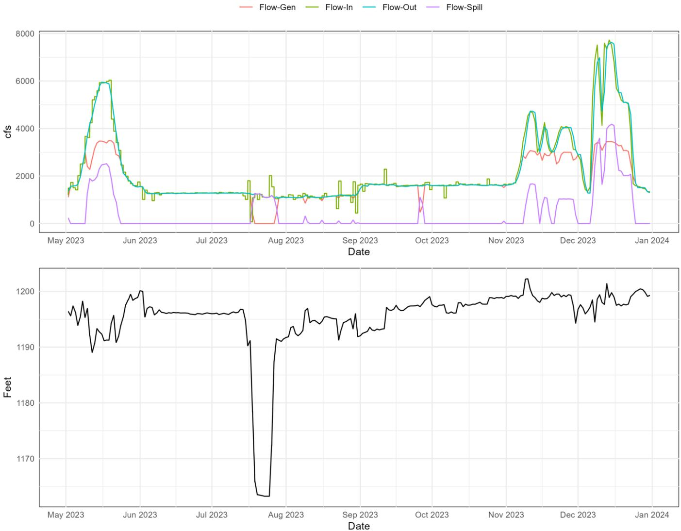
**Figure 15.** Dam operations at Big Cliff Dam. Top panel presents flow through the powerhouse (Flow-Gen), flow into the reservoir (Flow-In), flow out of the reservoir (Flow-Out), and flow through the spill gates (Flow-Spill). The bottom panel presents the forebay elevation.
