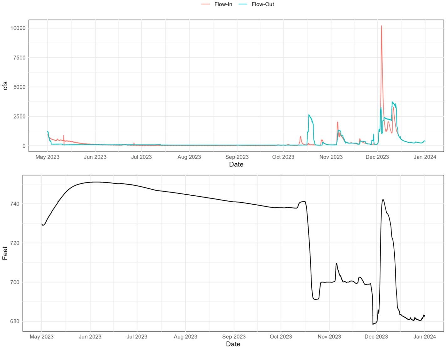
**Figure 11.** Dam operations at Fall Creek Dam. Top panel presents flow into the reservoir (Flow-In) and flow out of the reservoir (Flow-Out). The bottom panel presents the forebay elevation.
