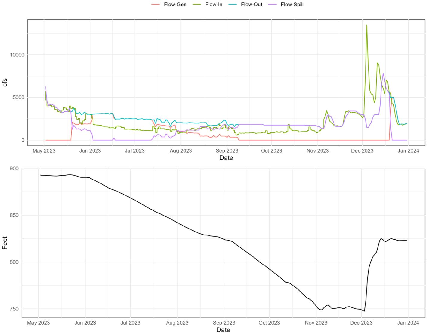
**Figure 10.** Dam operations at Lookout Point Dam. Top panel presents flow through the powerhouse (Flow-Gen), flow into the reservoir (Flow-In), flow out of the reservoir (Flow-Out), and flow through the spill gates (Flow-Spill). The bottom panel presents the forebay elevation.
